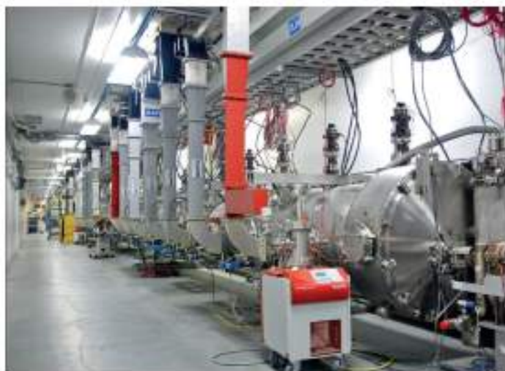
Fig. 2.11. CEBAF, a 12 GeV (was operating at 6 GeV) recirculating SRF linac at Thomas Jefferson Accelerator Facility. On the right – SRF accelerating modules. Upgrade to be finished by 2015.
