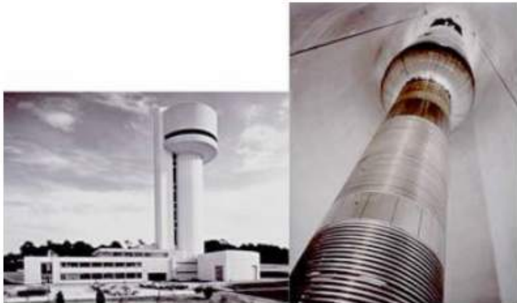
Fig. 2.4. Idea of the Van de Graaff invented an electrostatic generator and one of the biggest tandem accelerators at Daresbury (UK) with 42 m (14 stories high) 20 MV acceleration tube, placed vertically (Photo: CCLRC).
