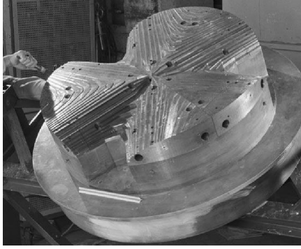
Fig. 1.14 Azimuthal pole shaping in Thomas-style AVF cyclotron.
