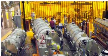
CEBAF, a 12 GeV recirculating SRF linac at Thomas Jefferson Accelerator Facility. On the right and the bottom – SRF accelerating modules.
