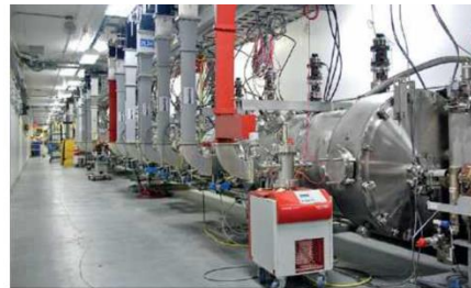
CEBAF, a 12 GeV recirculating SRF linac at Thomas Jefferson Accelerator Facility. On the right and the bottom – SRF accelerating modules.
