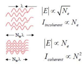
The positive feedback loop between radiation field and electron density bunching is the underlying mechanism of high gain FEL regime.
