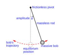
$$H = \frac{1}{2}h\omega_0\eta\delta^2 + \frac{eV\omega_0}{2\pi\beta^2 E_0}(\cos\phi - 1) \qquad H = \frac{1}{2}mv^2 + mgl(1 - \cos\phi)$$
