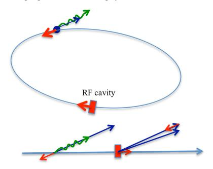
How radiation cools beam in a storage ring: vertical motion: Particle radiate in the direction of the motion and RF cavity restores only longitudinal part of the momentum.
