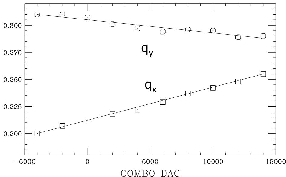
The fractional parts of betatron tunes were  $q_x = 4 - v_x$  and  $q_y = 5 - v_y$ . The experimental result of fractional horizontal tune appeared to “increase” with the strength of the quadrupole.
