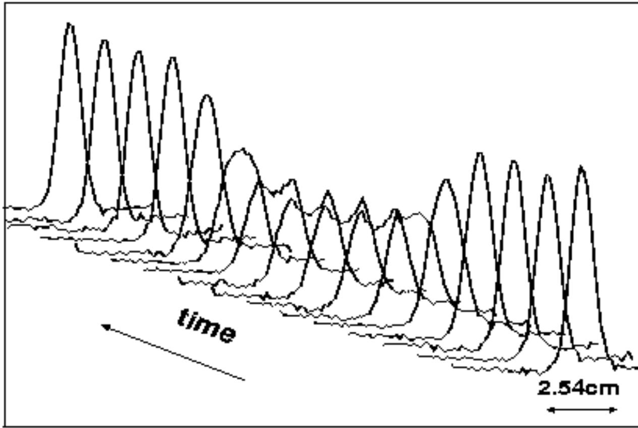
The beam profile measured from an ionization profile monitor (IPM) at the AGS during the adiabatic turn-on/off of an rf dipole. The beam profile appeared to be much larger during the time that the rf dipole was on because the profile was an integration of many coherent synchrotron oscillations. After the rf dipole was adiabatically turned off, the beam profile restored back to its original shape (@RHIC BNL).
