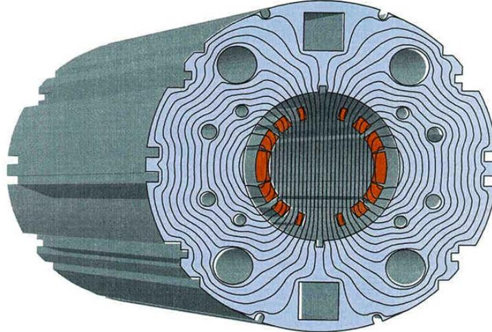
Typical super-conducting dipole magnet with  $\cos(\theta)$  coil (red). Current distribution approximates the  $\cos(\theta)$  with as many as possible high harmonics (sextupole, etc.) being compensated.
