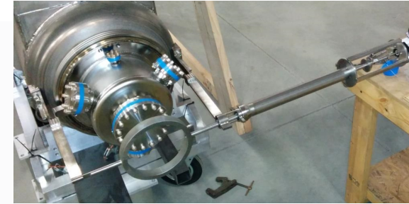
Dial Indicators for Deflection Measurements
