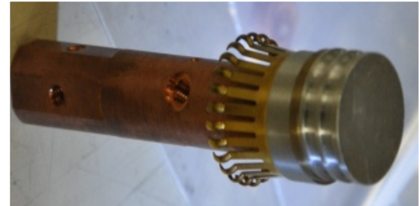
Photocathode end assembly
