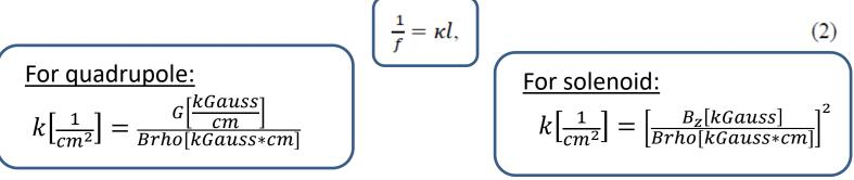
here  $\kappa$  is the magnet focusing strength in units of 1 over length squared and l is the effective length of the magnet.
