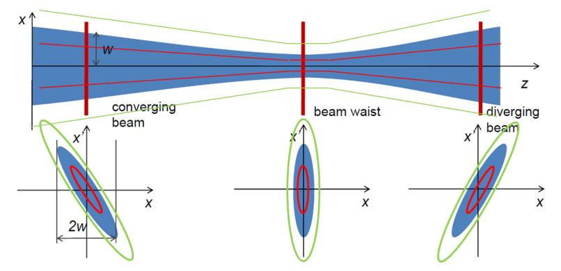
Along a beamline the orientation and aspect ratio of the beam ellipse in x, x' changes, but area (emittance) remains constant.
