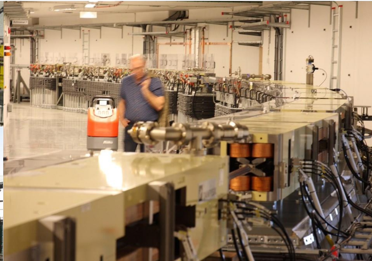
Two complete 7-bend achromats at MAX IV
