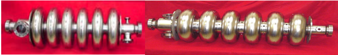
SNS 805 MHz cavities ( b = 0.61 and 0.81 )
