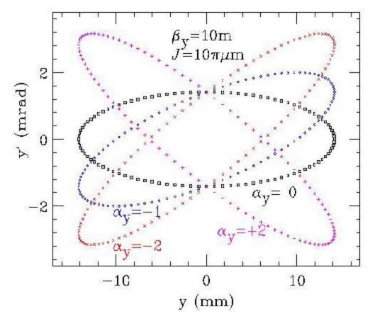
The betatron phase space ellipses of a particle with actions J =  $10\pi$  mm-mrad. The btatron parameters are  $\beta_y = 10m$ , and  $\alpha_y$  shown by each curve. The scale for the ordinate y is mm, and y' in mrad. The betatron parameters for each ellipse are marked on the graph. All ellipses has the maximum y coordinate at  $(2\beta_y J)^{1/2}$ . The maximum anglular coordiante y' is  $(2(1 + \alpha_y^2)J/\beta_y)^{1/2}$ . All ellipses have the same phase space area of 2J.
