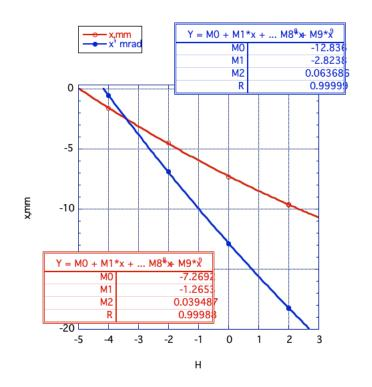
Measured dependence of horizontal position and angle as function of H (laser spot) at V=2 mm
