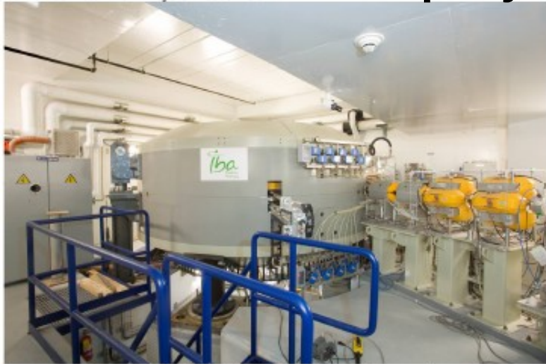
Figure 2. IBA 230 MeV resistive cyclotron for proton therapy
