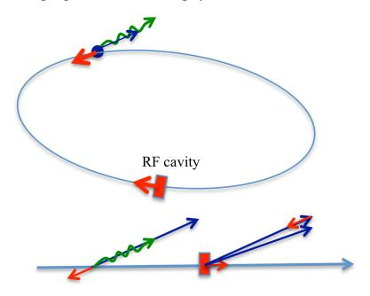
How radiation cools beam in a storage ring: vertical motion: Particle radiate in the direction of the motion and RF cavity restores only longitudinal part of the momentum.
