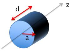
(b) We need to integrate on 3 surfaces: front and back faces (circles with radius a) and a cylinder of radius a and length d. Reversing the relations, 20 MV/m is equivalent to B=667 Gs. Corresponding  $H_o$ =5.31  $10^4$  A/m.
