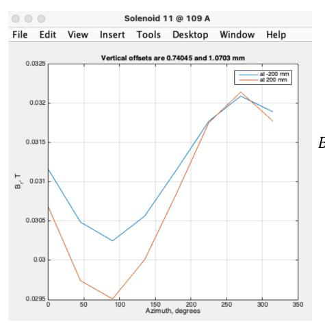
Vertical offsets are consistent with on axis fields (position -0.79 mm angle -0.55 mrad)
