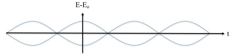
• When synchronous particles gaining or losing energy, topology of the phase space changes: particles can cross from the upper part to the bottom part (typical for qn acceleration or a energy loss case) or from the bottom to top (for a deceleration case) – these particles will be lost by hitting energy acceptance of the lattice  $E-E_0$
