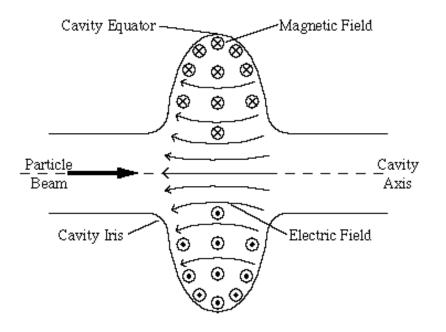
$$t = t_o + \frac{S}{V}; \Delta \mathbf{E} = eV_{RF} \sin(\phi + \phi_s); \quad \phi = \omega t_o$$
