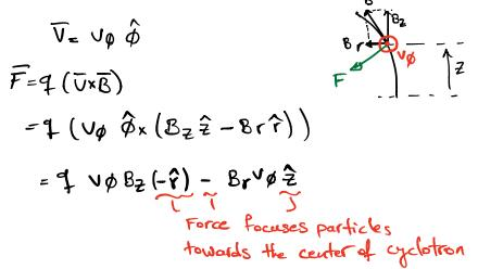
Note that at higher radius, the field lines become farther apart (I.e. the strength of field decreases), and therefore the focusing is achieved at the expense of the cyclotron force and frequency.
