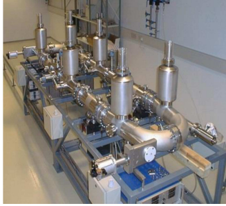
Fig. 1.7 Elisa in Aarhus, a 25 keV, 7.6 m circumference racetrack for molecular and atomic physics [9]. Its lattice combines spherical deflectors, plane deflectors and quadrupoles
