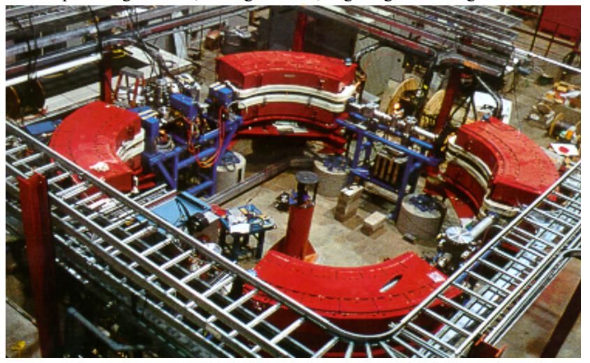
eCIS: No constraint on circumference (C=20m). Use CIS dipoles & cavity Need Damping wigglers, chicane, electrostatic kickers & septum
