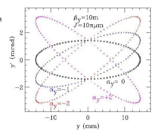
The betatron phase space ellipses of a particle with actions  $J=10\pi$  mm-mrad. The btatron parameters are  $\beta_y=10m$ , and  $\alpha_y$  shown by each curve. The scale for the ordinate y is mm, and y' in mrad. The betatron parameters for each ellipse are marked on the graph. All ellipses has the maximum y coordinate at  $(2\beta_yJ)^{1/2}$ . The maximum anglular coordinate y' is  $(2(1+\alpha_y^2)J/\beta_y)^{1/2}$ . All ellipses have the same phase space area of 2J.
