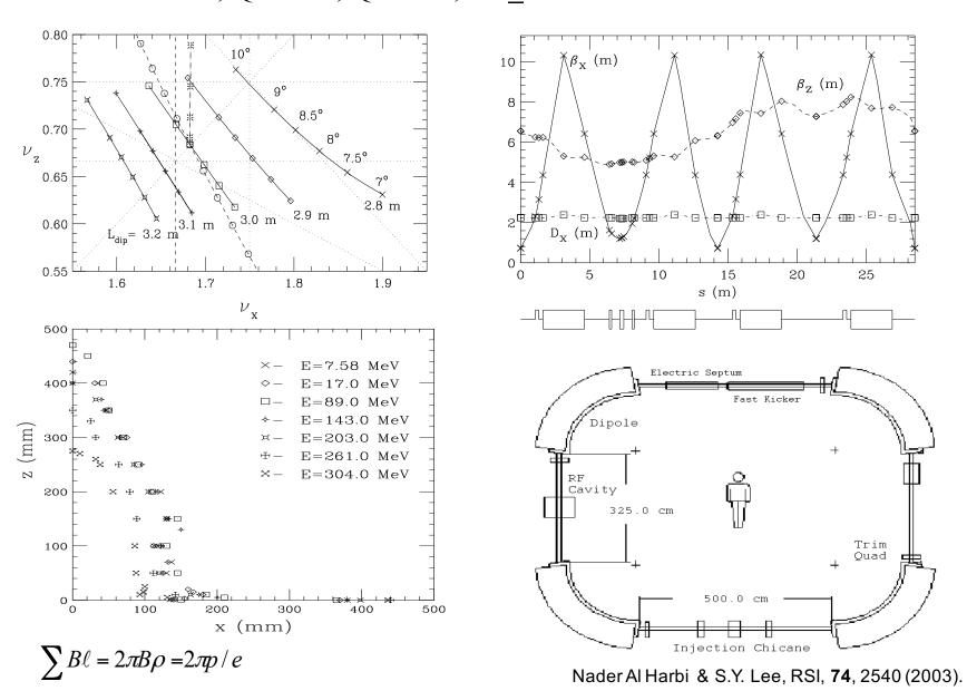
Low energy synchrotrons often rely on the bending radius  $K_x=1/\rho^2$  for horizontal focusing and edge angles in dipoles for vertical focusing. Find the lattice property of the low energy synchrotron described by the following input data file (MAD). What is the effects of changing the edge angle and dipole length? Discuss the stability limit of the lattice.
