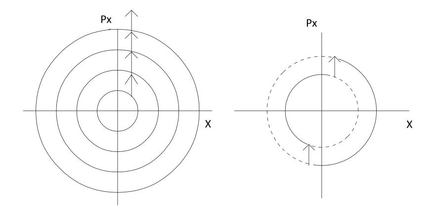
Left, a schematic plot of the closed-orbit perturbation due to an error dipole kick when the betatron tune is an integer. Here  $p_X = \beta_X \Delta X' = \beta_X \theta$ , where  $\theta$  is the dipole kick angle and  $\beta_X$  is the betatron amplitude function value at the dipole. Right, a schematic plot of the particle trajectory resulting from a dipole kick when the betatron tune is a half-integer; here the angular kicks from two consecutive orbital revolutions cancel each other.
