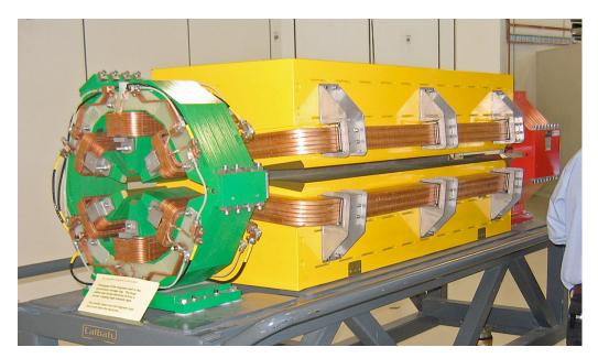
Typical elements of accelerators are dipoles and quadrupoles (or their combination), sextupoles and octupoles (they a nonlinear), solenoids, wigglers.... Let's start from a linearized Hamiltonian (143) magnetic DC elements – this is typical accelerator beamline.
