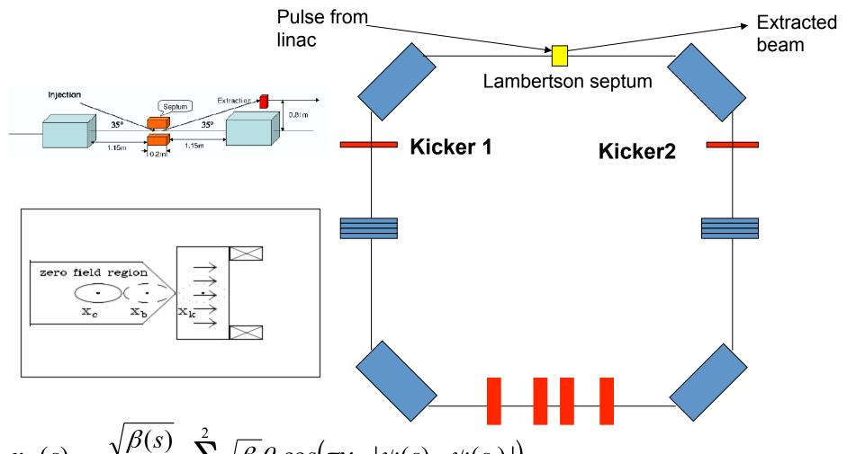
$$x_{co}(s) = \frac{\sqrt{\beta(s)}}{2\sin(\pi v)} \sum_{i=1}^{2} \sqrt{\beta_i} \theta_i \cos(\pi v - |\psi(s) - \psi(s_i)|)$$
